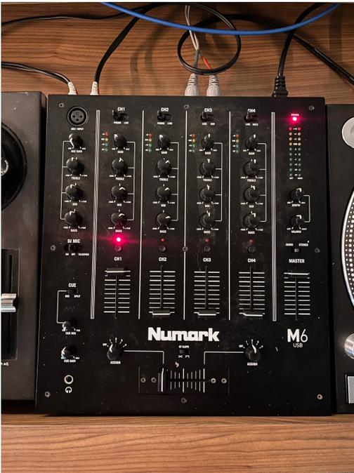
There is a large fader for each player. The left turntable's level is controlled by the left half of controls, and vice versa for the right turntable.
